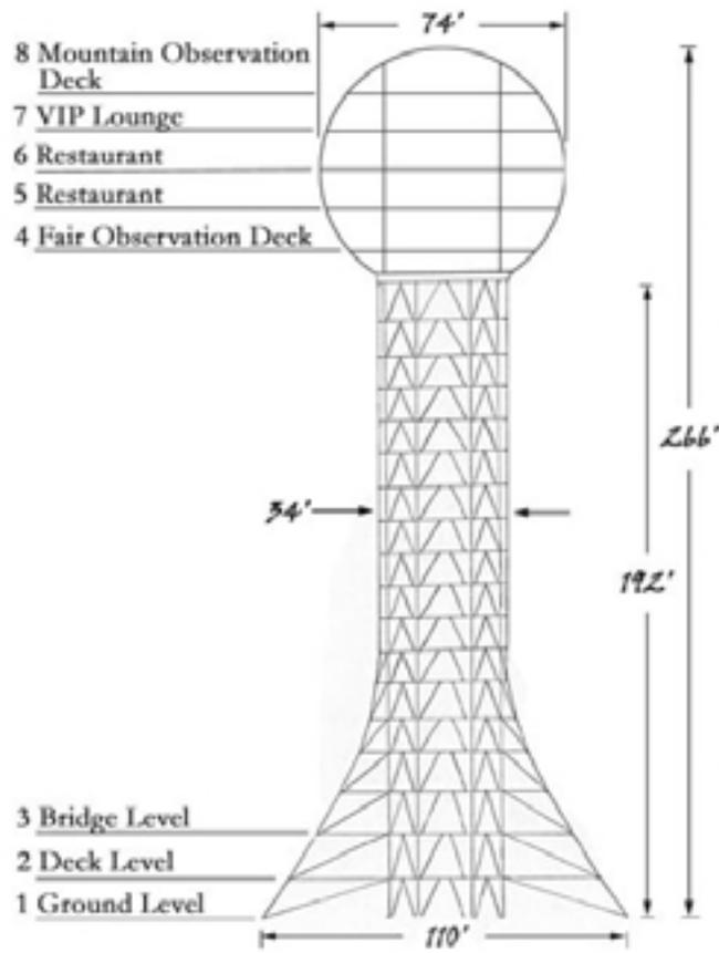
Figure 6: A schematic drawing of the Sunsphere.
